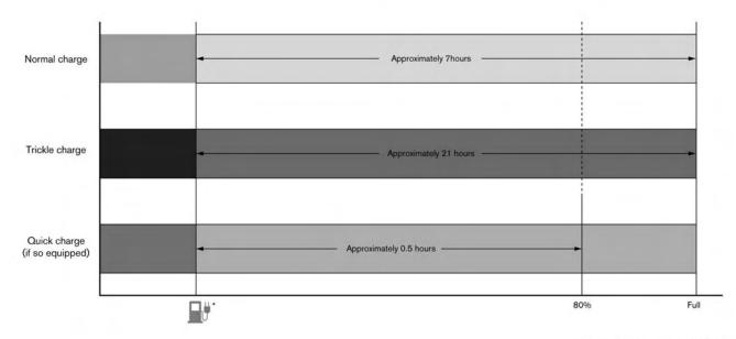
\*: Low battery charge warning light is ON.
