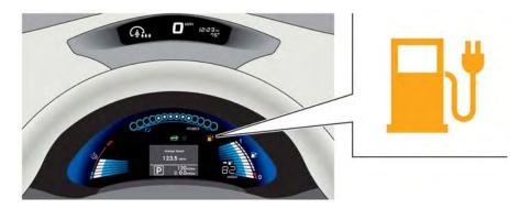
If the low battery charge warning light **I** illuminates, the Li-ion battery charge is too low for travel. See "Low battery charge warning light" in the "2. Instruments and controls" section. Charge the Li-ion battery as soon as possible.
