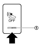
The Approaching Vehicle Sound for Pedestrians (VSP) system is a function that uses sound to help alert pedestrians of the presence of the vehicle when it is being driven at a low speed.
