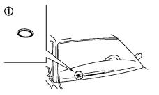
Be sure not to put anything on top of the photo sensor (1) located on the top of the instrument panel. The photo sensor controls the autolight; if it is covered, the photo sensor reacts as if it is dark and the headlights will illuminate.
