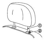
To lower, push and hold the lock knob and push the headrest down.
