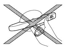
Do not pull the door handle before pushing the door handle request switch. The door will be unlocked but will not open. Release the door handle once and pull it again to open the door.
