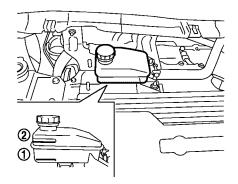
Check the fluid level in the reservoir. If the fluid is below the MIN line ① or the brake warning light illuminates, add Genuine NISSAN Super Heavy Duty Brake Fluid or equivalent **DOT 3** fluid up to the MAX line ②. If fluid must be added frequently, the system should be checked by a NISSAN certified LEAF dealer.
