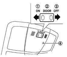
The map light control switch has three positions: ON (1), DOOR (2) and OFF (3). The light (4) (if so equipped) will illuminate when the headlight switch is turned to the  $\exists pd \exists$ or  $i \in D$  position.
