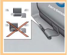
Pass the lower side belt of the EVSE (Electric Vehicle Supply Equipment) case securely through the fastener on the bottom of the luggage board. If the case suddenly becomes loose, it may cause serious injury or death.
