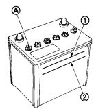
Check the fluid level in each cell. It should be between the UPPER LEVEL (1) and LOWER LEVEL (2) lines.
