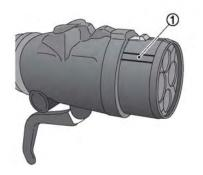
4. Align (1) with the groove of the charge port and insert the charge connector.
