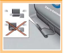
Pass the lower side belt of the EVSE (Electric Vehicle Supply Equipment) case securely through the fastener on the bottom of the luggage board. If the case suddenly becomes loose, it may cause serious injury or death.
