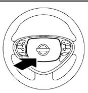
To sound the horn, push the center pad area of the steering wheel.
