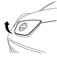
2. Put your hand into the under side of the lid and open until it is in the fully open position.
